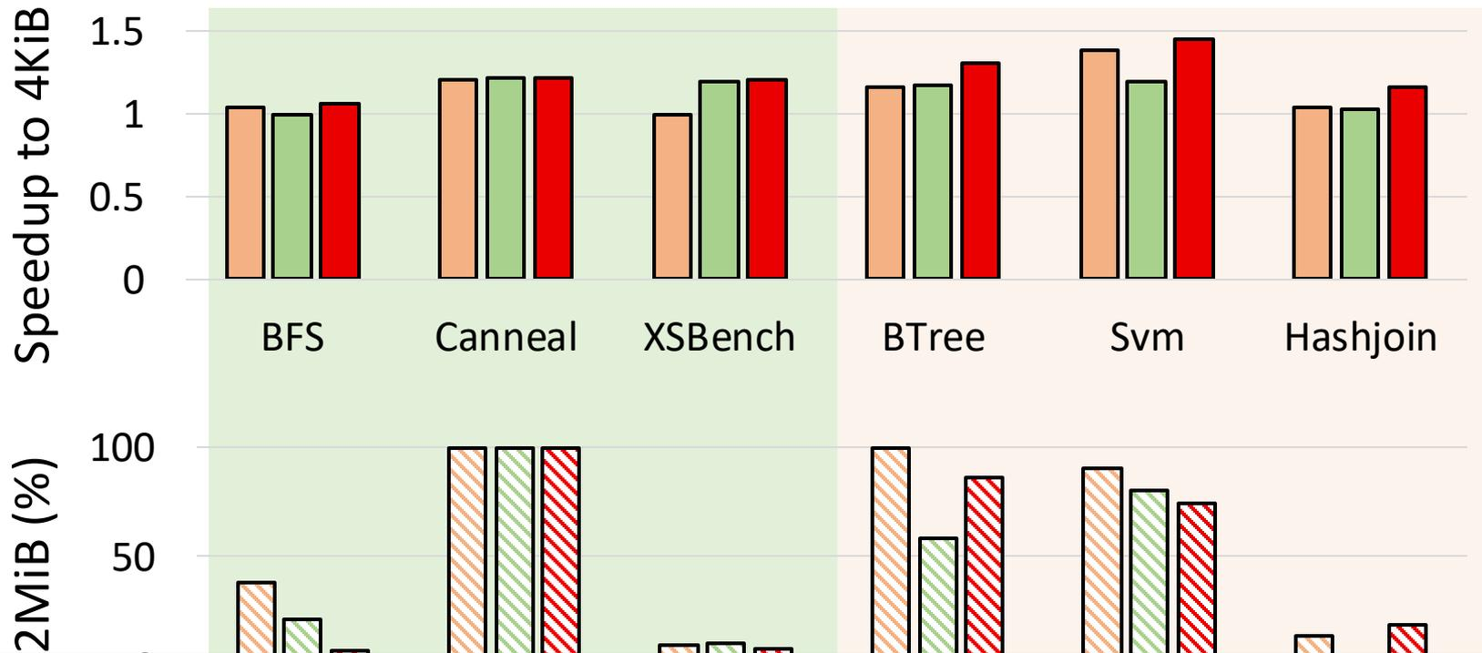
Leshy guidance allows ET to optimally use all translation sizes to boost performance by 10% on average while reducing 2MiB usage
